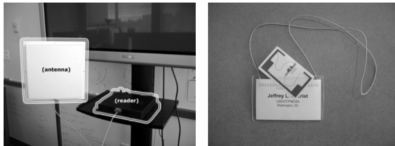
Fig. 1. (a) RFID tag reader (right) and antenna (left); (b) RFID tag and conference badge.
